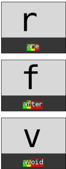
Figure 1: Suggestion per key is estimated with previous letters entered by user, and letter associated with the key as input. In the image above the already collected part of the word is framed green, the letter on the key as yellow, and the suggestive part by prediction engine red.
